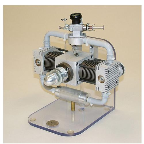
You can see the serrated drive belt and one of the pulleys for the rotary valves at the back of the engine.
